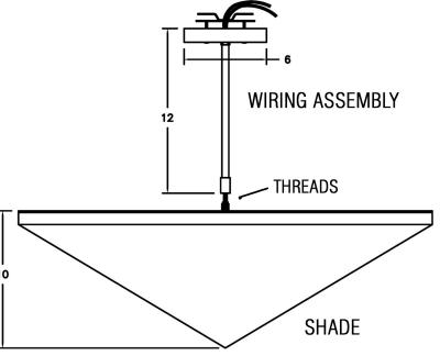
ATTACH WIRING ASSEMBLY TO EXPOSED THREADS ON SHADE ASSEMBLY MAKING SURE THAT ALL WIRES ARE THREADED THROUGH ROD AND CANOPY. ATTACH ASSEMBLED FIXTURE TO CEILING AS BELOW.
