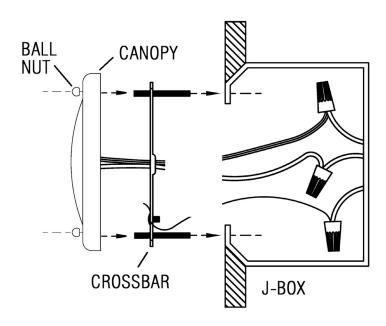
IMPORTANT TURN OFF THE POWER AT THE MAIN FUSE OR CIRCUIT BREAKER **BOX BEFORE** STARTING INSTALLATION
