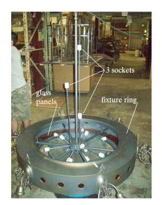
PLACE FIXTURE RING ONTO BARREL OR SAW HORSES CAREFUL PLACE GLASS PANELS INTO BOTTOM OF FIXTURE RING (MAKE SURE FLAT SIDE OF GLASS FACES DOWN) PLACE LIGHT BULBS INTO (3) SOCKETS
